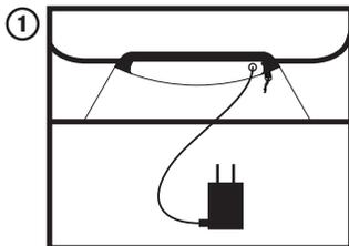
Feed the power cable through the rear power supply pocket.
