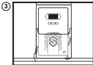
Secure the **OZ500** in the pocket then connect the power supply to the left side of the unit.
