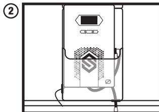
Connect plastic hose to orange elbow then connect elbow to the right side of the **OZ500**. Feed hose through bottom grommet of inner bag & connect to the nozzle inside the bag.
